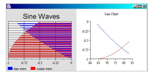
The same data feed drives both charts, with updates every second. However, the first chart is based on serialized information created with a BarChart bean customizer. Like all horizontal bar charts, the Y axis is horizontal. The LineChart bean used for the second chart uses the same data, but displays it on a vertical Y axis and horizontal X axis.
